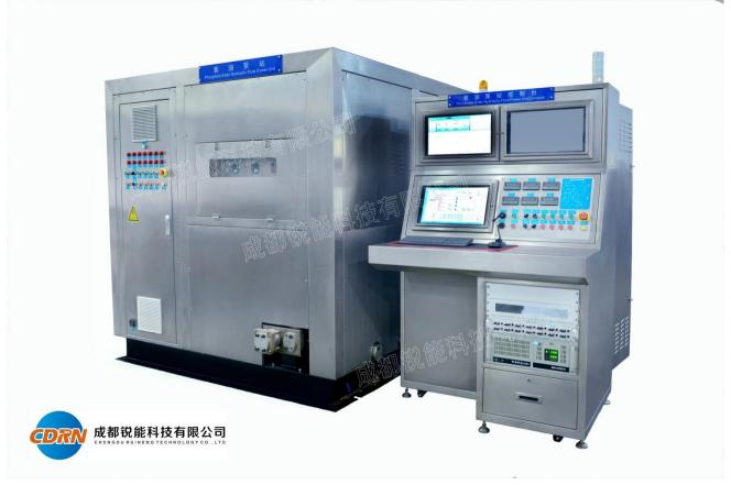
The hydraulic pump station mainly provides centralized hydraulic power source for all kinds of aircraft hydraulic finished parts test bench or other hydraulic equipment. According to the pressure requirements of different hydraulic equipment, it can provide two pressure levels of 3000PSI and 5000PSI, and can provide two working media of red oil and blue oil in accordance with the needs of the working medium of hydraulic finished parts.
